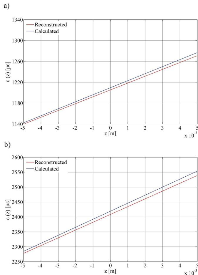
Fig. 6. Calculated strain profile and reconstructed strain profile: a)  $\varepsilon(z) = 1209\mu\varepsilon + (13.44\mu\varepsilon/\text{mm})z$ ;
