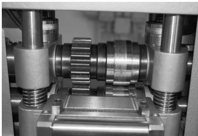
Fig. 2. Toothed and flat rolls for RCS process
