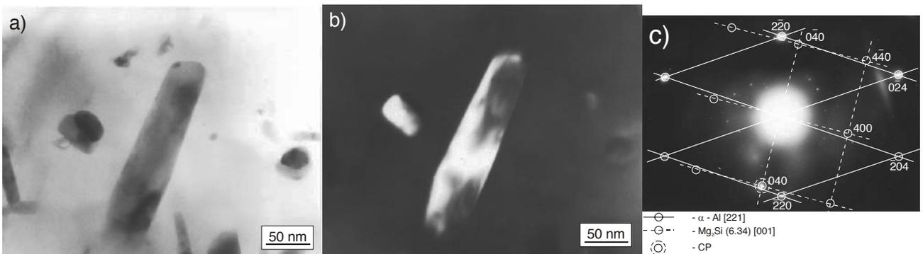
Fig. 11. TEM micrograph of C355.0 alloy in T6 conditions showing the precipitate of the  $\beta$ -Mg<sub>2</sub>Si phase (a,b), and corresponding electron diffraction pattern (c)
