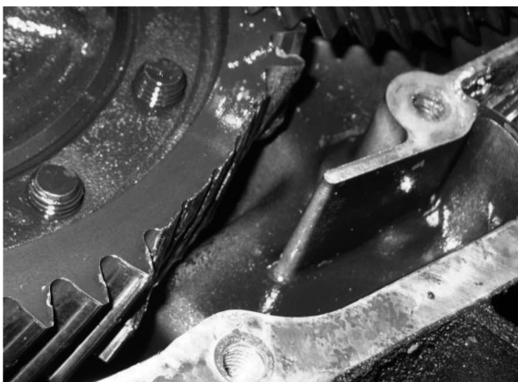
Fig. 15. Defected toothed wheels of main shaft
