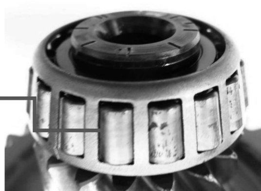
Fig. 11. Damaged roller element
