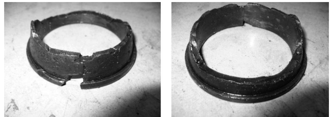
Fig. 16. Totally damaged inside track of roller bearing in lorry
