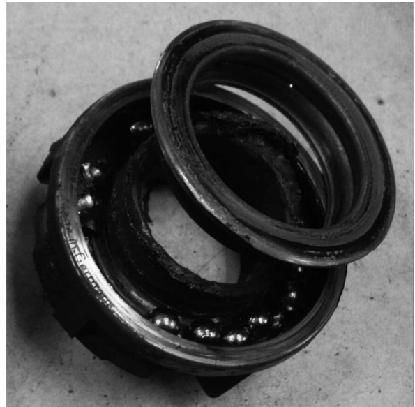
Fig. 7. Worn thrust bearing
