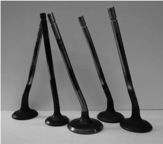
Fig. 5. Distortion of valves
