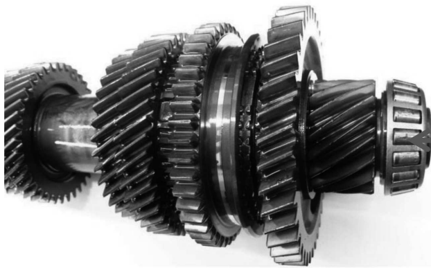
Fig. 10. Main shaft of gearbox and damaged tapered roller bearing
