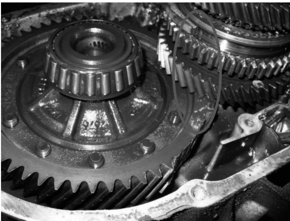
Fig. 14. Damaged bearing of main shaft
