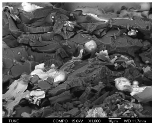
Fig. 9. Al 2 O 3 coating sandwich structure on the fracture area
