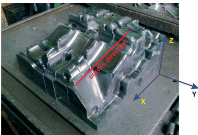
Fig. 4. Coordinate system orientation with respect to direction of surface cracks (red line)
