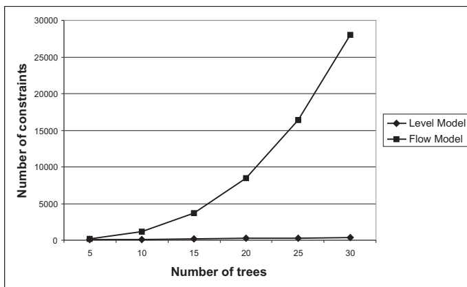
Fig. 3. Number of constraints as a function of the number of trees and the type of approach (8 levels, 11 link types).
