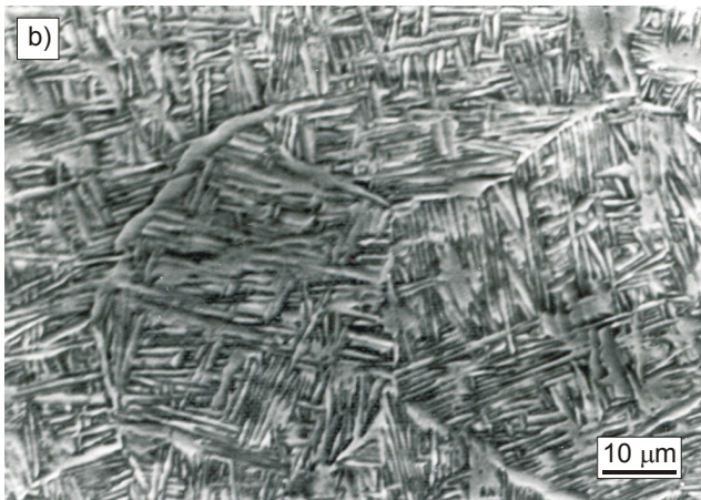
Fig. 5. Remelted zone, a) the grain boundaries of prior \alpha phase is visible, b) bottom structure of RZ
