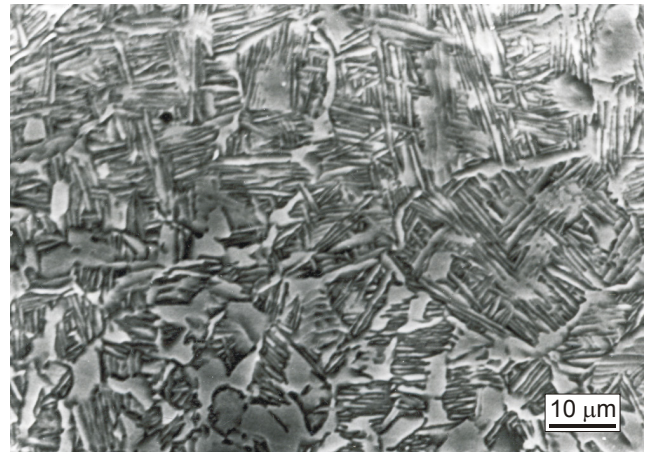
Fig. 6. Microstructure on the border RZ and HAZ
