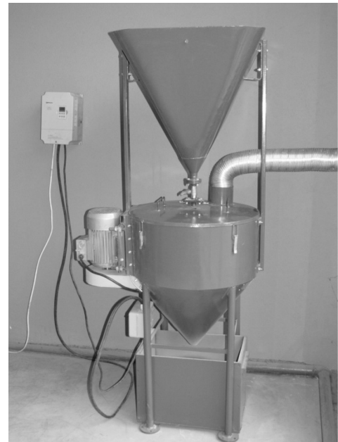
Fig. 4. General view of tribotester 9-Bitter [7]
