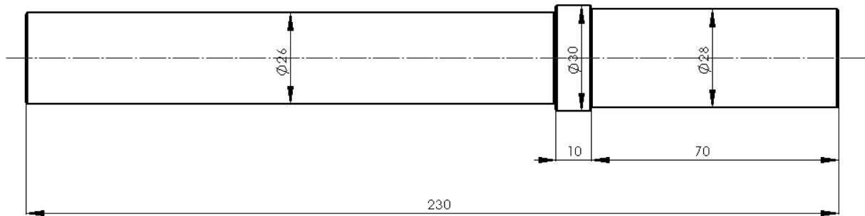
Fig. 2. Shape and dimensions of antenna
