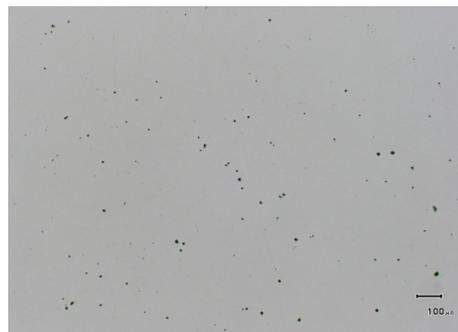
Fig. 7. Complex oxisulphides of rare earth metals (1,000 x)
