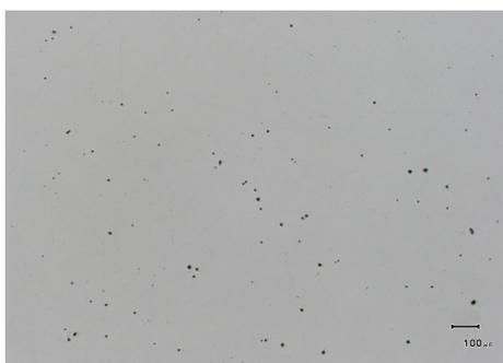
Fig. 5. Globular inclusions after deoxidation with Al+Ti (100 x)
