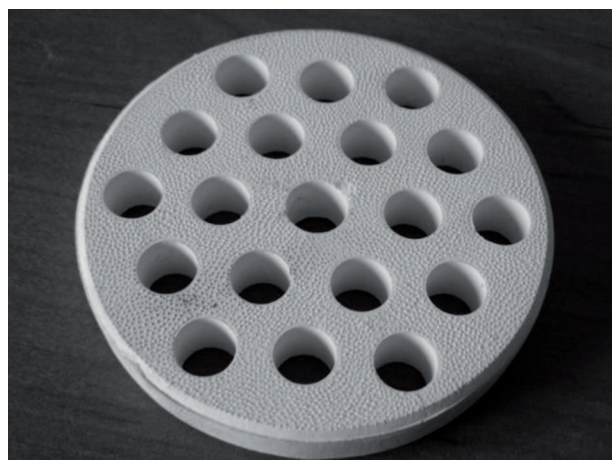
Fig. 3. Multi-hole ceramic filter
