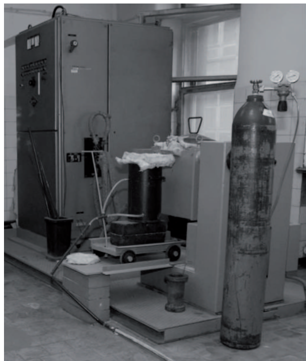
Fig. 2. Position for process of steel filtrati in the atmosphere of argon
