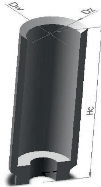
Fig. 1. The product deep sleeve, where: H_c – total height, D_w – internal diameter, D_z – outside diameter
