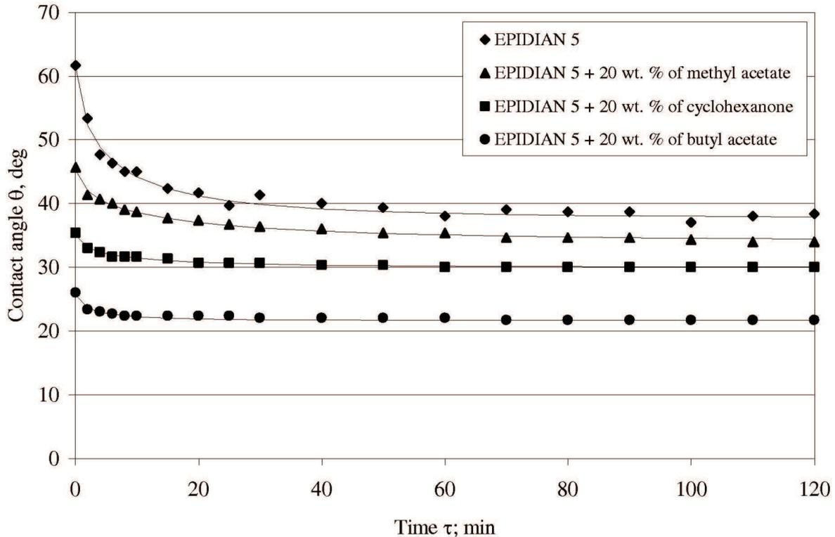
Fig. 1. Time-related changes in the contact angle  $\theta$  in a quartz – EPIDIAN 5 + diluent system; SEP – 62,7 mJ/m<sup>2</sup>; t = 10°C = const
