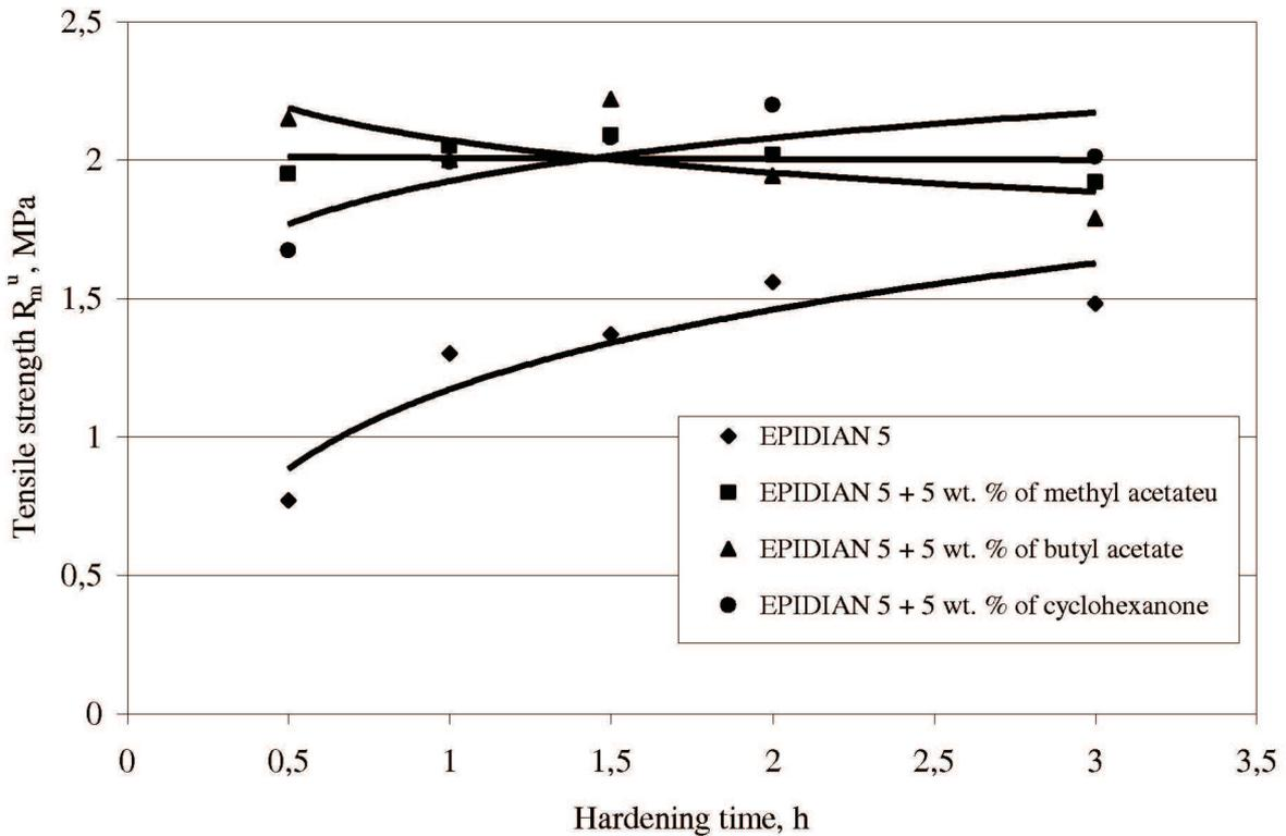
Fig. 2. Effect of hardening time on the tensile strength  $R_m^u$  of sand with an addition of binder: EPIDIAN 5 resin; EPIDIAN 5 + 5 wt.% methyl acetate, EPIDIAN 5 + 5 wt.% butyl acetate, EPIDIAN 5 + 5 wt.% cyclohexanone. Mixing conditions: 1) sand + binder 1,5 min, 2) sand + binder + hardener – 1,5 min, sand compacted by vibrations, hardening temperature – 100°C
