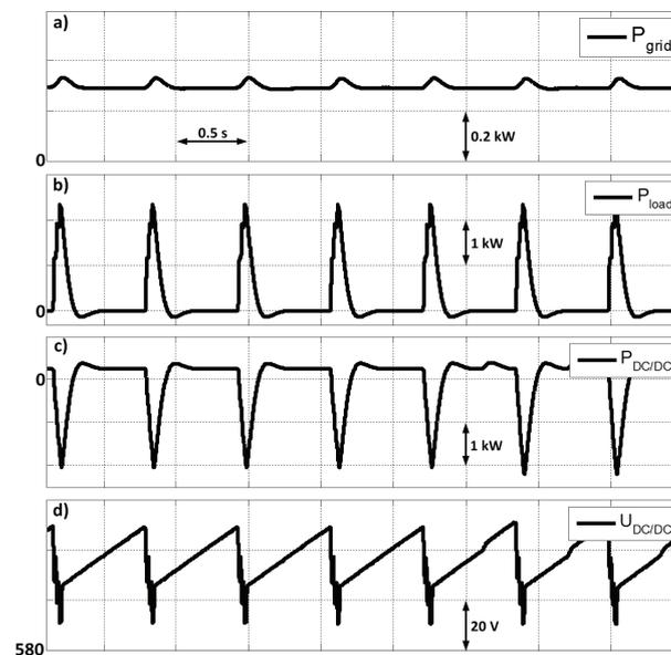
Fig. 10. Active power waveforms recorded in selected system points: a) drawn from the feed line; b) drawn by the load; c) circulating in the DC-DC converter circuit; d) voltage  $U_{DC/DC}$  on the DC-DC converter capacitor
