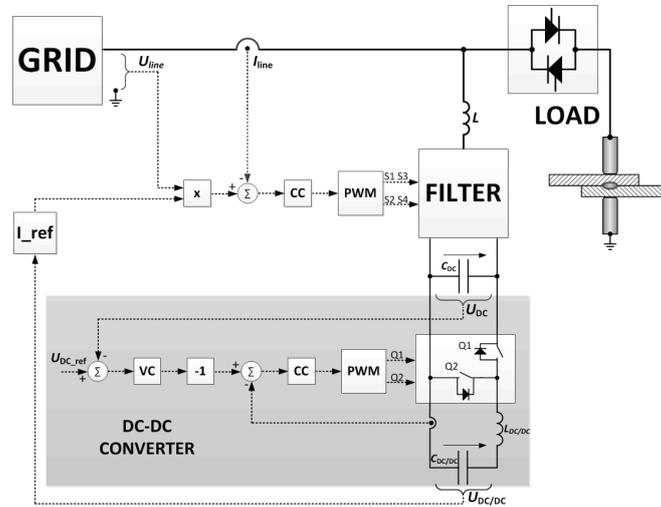
Fig. 2. Block diagram of the filter system with additional energy storage and control system; where:
