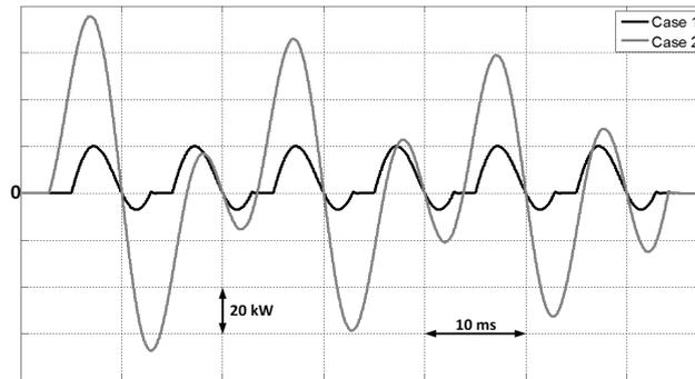
Fig. 8. Momentary active power value waveforms during welding
