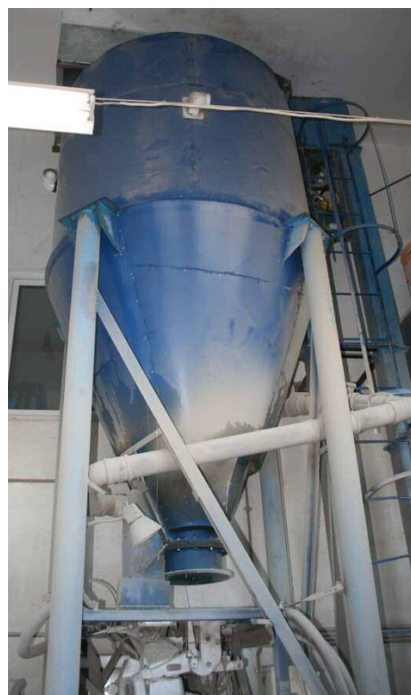
Fig. 2. Mixing line in the following unit: a feed mixer, an intake hopper and a bucket conveyor
