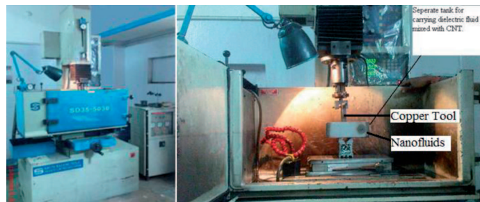
Fig. 2. EDM machine with nanofluids and electrode setup
