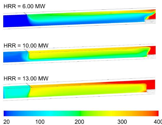
Fig. 16. Temperature plot ( $20\text{--}200^\circ\text{C}$ ) for proximity of air curtain and the source of fire, for  $U_o = 10 \text{ m/s}$ ,  $I = 0.5\%$ ,  $\alpha = 30^\circ$ , HRR = 6.0 MW, 10.0 MW, 13.0 MW
