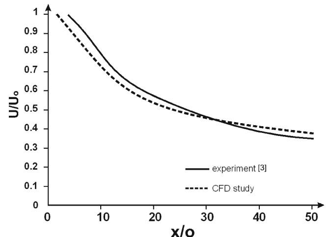
Fig. 5. Results of centreline velocity decay, for  $U_o = 27$  m/s,  $I = 0.5\%$ ,  $\alpha = 0^\circ$  [5]
