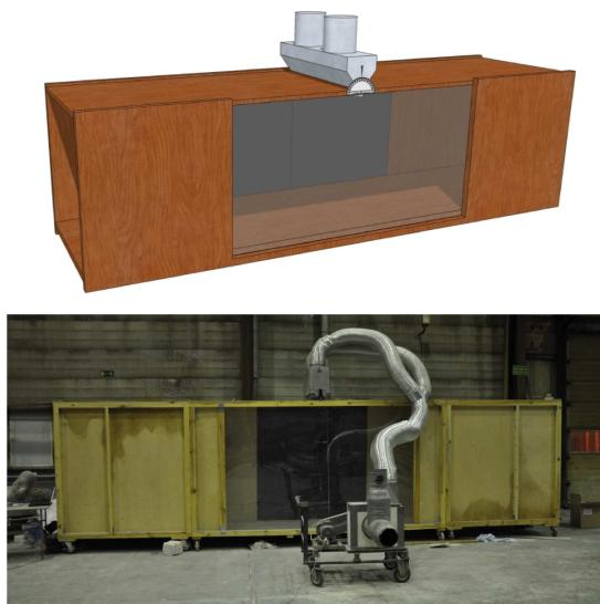
Fig. 8. Scheme (up) and a photography (down) of the test tunnel facility (Ref. 19)
