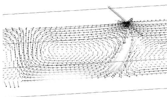
Fig. 18. Velocity vectors at the proximity of air curtain (0–5 m/s) for  $U_o = 10 \text{ m/s}$ ,  $I = 0.5\%$ ,  $\alpha = 30^\circ$ , HRR = 13.0 MW, fire on the right side of air curtain
