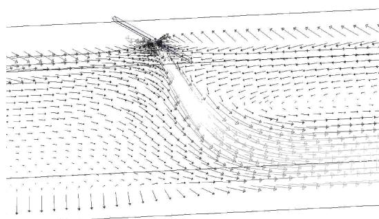
Fig. 17. Velocity vectors at the proximity of air curtain (0–5 m/s) for  $U_o = 10 \text{ m/s}$ ,  $I = 0.5\%$ ,  $\alpha = 30^\circ$ , HRR = 6.0 MW, fire on the right side of air curtain
