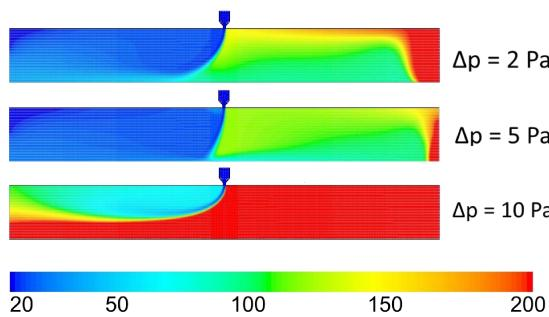
Fig. 15. Temperature plot, for  $U_o = 10 \text{ m/s}$ ,  $I = 0.5\%$ ,  $\Delta p = 3.5$  and  $10 \text{ Pa}$ ,  $\alpha = 0^\circ$
