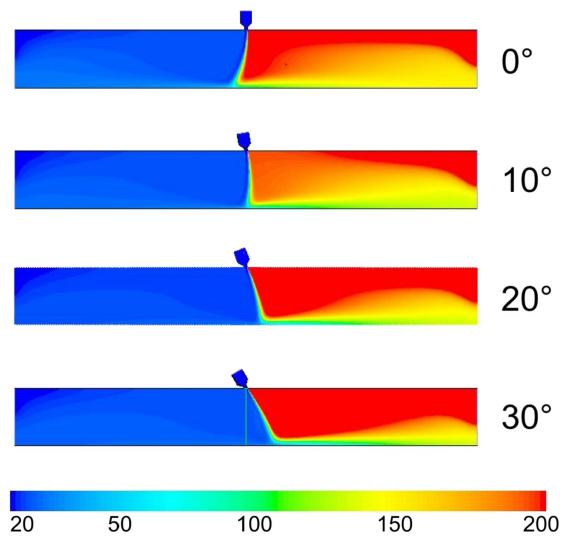
Fig. 20. Temperature plot ( $20\text{--}200^\circ\text{C}$ ), for  $U_o = 30 \text{ m/s}$ ,  $I = 0.5\%$ ,  $\Delta p = 10 \text{ Pa}$ ,  $\alpha = 0^\circ$ ,  $10^\circ$ ,  $20^\circ$  and  $30^\circ$
