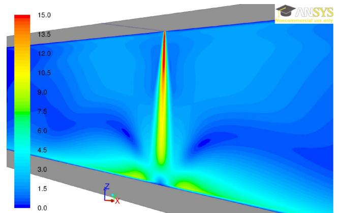
Fig. 6. Contours of velocity (0–15 m/s), for  $U_o = 27$  m/s,  $I = 0.5\%$ ,  $\alpha = 0^\circ$ , realizable  $k-\varepsilon$  turbulence model [5]
