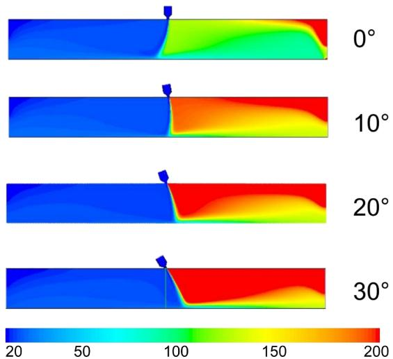
Fig. 19. Temperature plot ( $20\text{--}200^\circ\text{C}$ ), for  $U_o = 20 \text{ m/s}$ ,  $I = 0.5\%$ ,  $\Delta p = 10 \text{ Pa}$ ,  $\alpha = 0^\circ$ ,  $10^\circ$ ,  $20^\circ$  and  $30^\circ$
