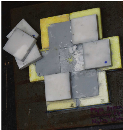
Fig. 6. Images of ballistic test results (7.62×54R AP, 1 round) for the A1T (a) and C1T (b) developed armour systems
