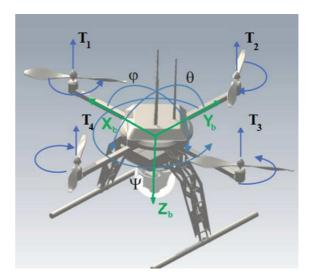
Fig. 5. Conceptual drawing of a simulated quadrotor
