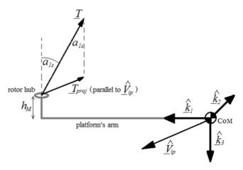
Fig. 3. Thrust vector deflection caused by flapping
