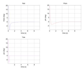
Fig. 6. Attitude angles evolution of hover flight with initial 20 degrees misalignment in every axis
