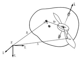
Fig. 2. Geometry of quadrotor with rotor incorporated into the model
