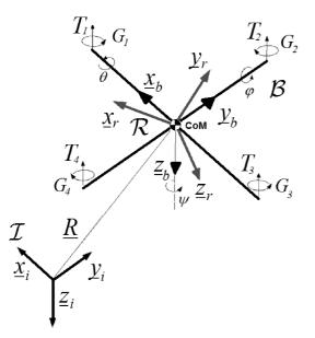
Fig. 1. Reference frames used together with principal axes, forces and moments
