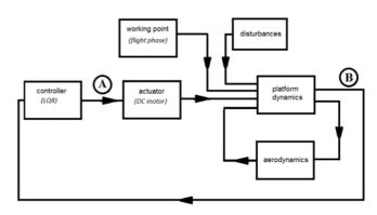
Fig. 4. Schematic of a control system, where part between A and B is linearized for LQR design
