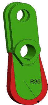
Fig. 18. Example of optimization of the crank shape in the drive system
