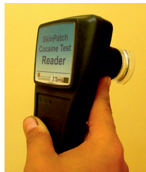
Fig. 13. Lab-on-a-paper – based test for detection of cocaine: a) scheme of the measurement setup for, b) view of the hand-held reader co-working with the test
