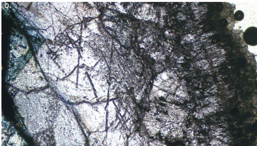
Text-fig. 8b. The same field of view as Text-fig. 8a but under PPL (plain polarized light) and stained. Zone B stains as non-ferroan calcite (pink), Zone C stains as ferroan calcite (blue)
