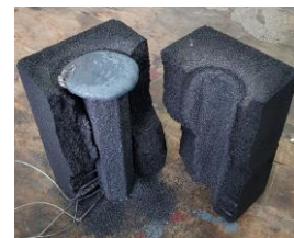
Fig. 11. A cast sample for the analysis of the cooling rate as a function of the distance from the surface of the cooling plate, with the view of the positioning of the thermocouples
