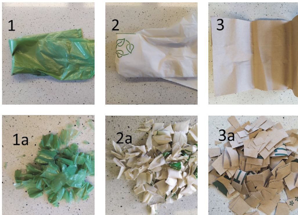
Fig. 1. Tested materials 1–1a. Oxy, 2–2a. Corn, 3–3a. Pap before and after shredding (photo: Biernacki, M.)
