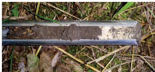
Fig. 2. An exemplary sample, taken with an Egner's cane (photo by Ł. Gawor)
