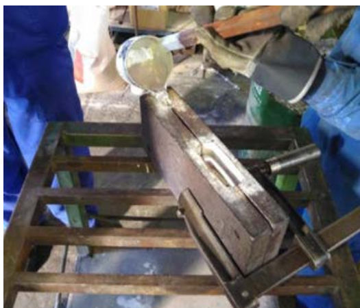
Fig. 1. The gravity casting procedure of initial samples
