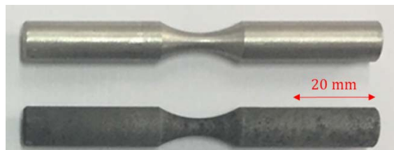
Fig. 4. Fatigue test samples, including before (the above one) and after (the bottom one) the pre-corrosion process
