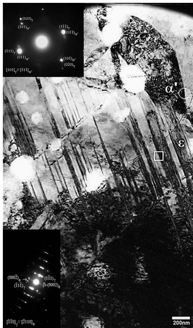
Fig. 3. Bright field TEM image and electron diffraction patterns obtained from the selected areas (interfaces) for sample A
