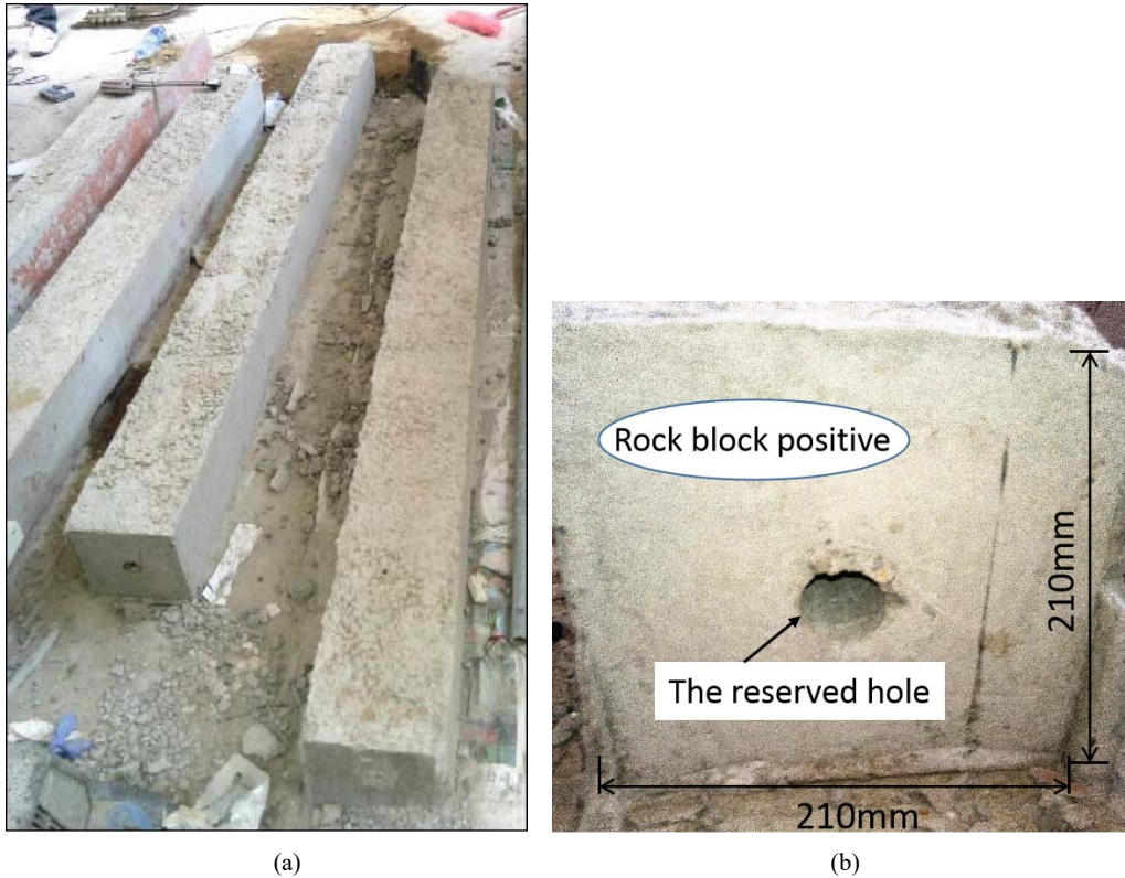
Fig. 2. Surrounding rock specimen. (a) Overall picture of rock mass; (b) Cross section of rock specimen
