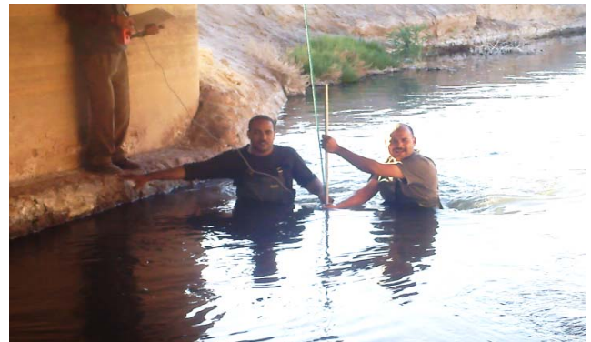
Photo 4. Flow velocity measurements at the centre of the canal (phot. M. Sayah Lembarek)
