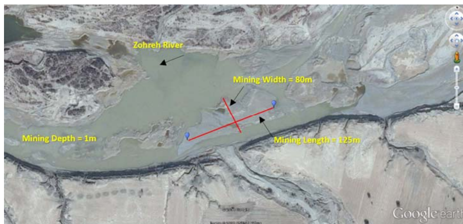
Fig. 6. Geometrical dimensions of the sedimentary deposit considered for material mining along the Zohreh River; source: own elaboration
