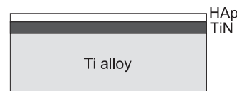
Fig. 1. Scheme of multilayer with improved biocompatibility material comprising TiN interlayer obtained by glow discharge nitriding and HAp outer layer deposited by PLD
