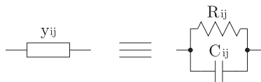
Fig. 2. General form of admittance element of filter in Fig. 1 (here for y_{ij} )
