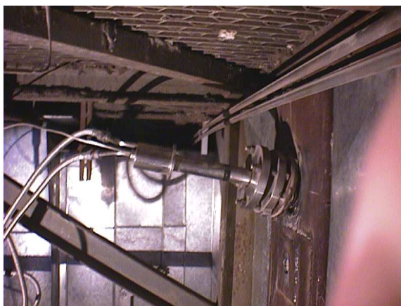
Fig. 5. The optical fibre probe with optoelectronic block
