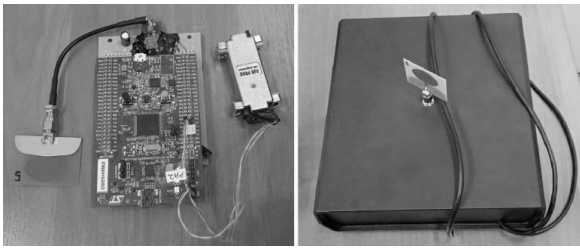
Fig. 1. UWB environment – tag for data acquisition (left), an anchor serves as a station (right)
