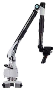
Fig. 1. A Romer Absolute 7520si measuring arm.
