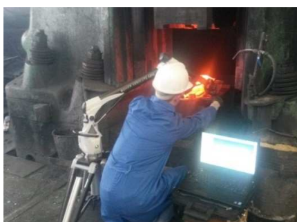
Fig. 20. Measurements of a "hot" forging of a scraper (the indirect reverse scanning method) and a forging die on a hammer, during a technological break (in order to verify the reverse method).
