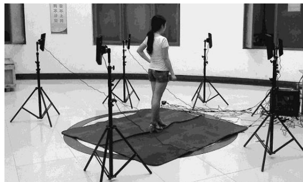
Fig. 6. Human body reconstruction via multiple low-cost depth cameras [14].
