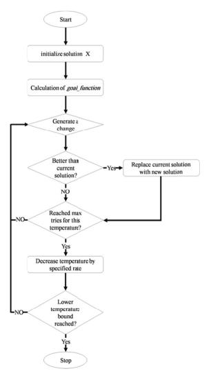
Fig. 4. Simulated annealing algorithm
