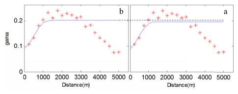
Fig. 3. Models fitted to the experimental variogram: a) with the Cressie weighting relation and, b) with the modified relation
