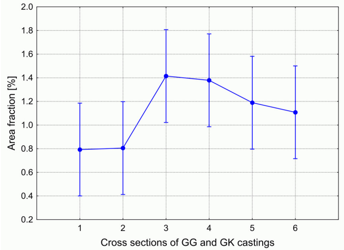
Fig. 10. Comparison of area fraction of (\gamma + \gamma') eutectic areas between the cross sections of GK and GG cast jointly
