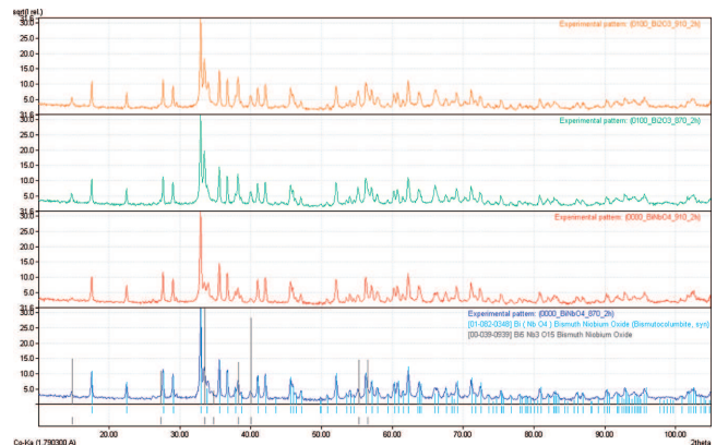
Fig. 3. Comparison of X-ray diffraction patterns of \text{BiNbO}_4 ceramics with diffraction lines positions of major ( \alpha\text{-BiNbO}_4 ) and minor ( \text{Bi}_5\text{Nb}_3\text{O}_{15} ) phases
