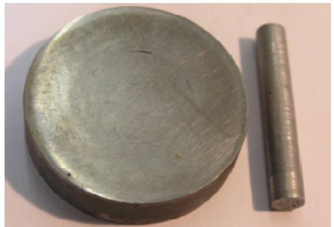
Fig. 1. Pin on disc contact used in tribological test (pin GJS-400, disc AlMC)
