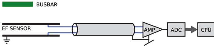
Fig. 4. A single measurement channel with EF sensor.
