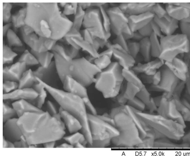
Fig. 2. Fracture of the preform made of the  $\alpha$ -Al<sub>2</sub>O<sub>3</sub> particles with the visible binding bridges
