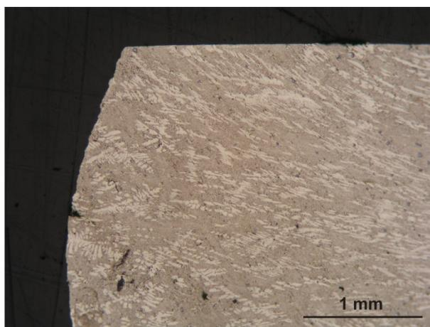
Fig. 6. The microstructure of an unreinforced material EN AC-4200 after deformation. Test temperature: 250°C
