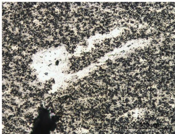
Fig. 8. The front of the slip crack and deformed regions without strengthening particles in the composite material EN AC-44200-20 vol. % Al<sub>2</sub>O<sub>3</sub>. Test temperature: 250°C
