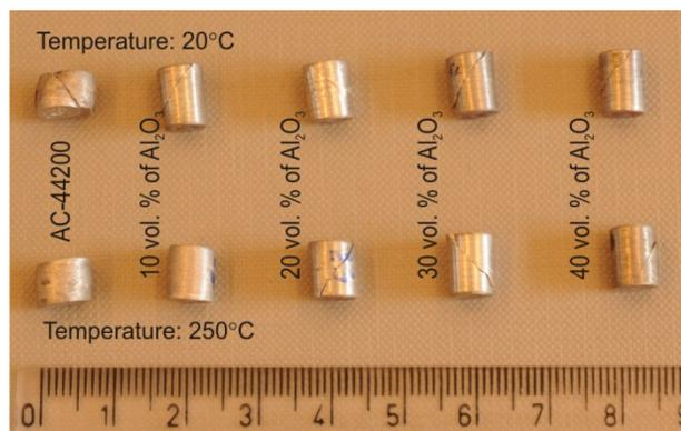
Fig. 4. Deformations of specimens after compression test at temperature: 20°C and 250°C
