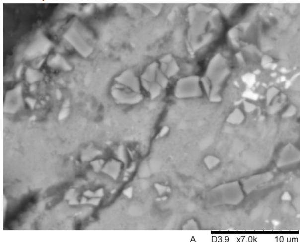
Fig. 11. SEM of a fracture of composite material EN AC-44200-10 vol.%  $\text{Al}_2\text{O}_3$ . Test temperature: 20°C
