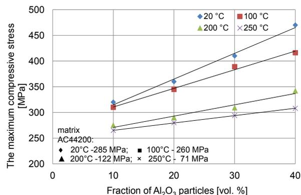
Fig. 5. Maximum compressive stress of EN AC-44200 alloy and composite materials
